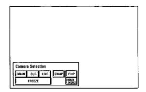
MAIN:selects picture shot by the Main CameraSUB:selects picture shot by the Sub CameraLINE:selects picture connected to the Line Input<br/>such as VCR.
