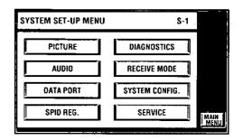
4. Move the high-lighted bar to the desired item by moving the Joystick then press the Joystick to execute the selection.
