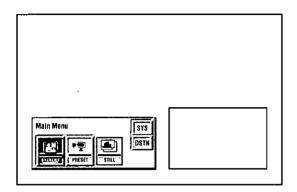
3. Move the high-lighted bar to the desired mode from MAIN; SUB, or LINE by moving the Joystick then press the Joystick to select desired picture.
