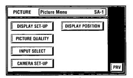
Move the high-lighted bar to the each item by moving the Joystick then adjust the camera by pressing the Joystick.
