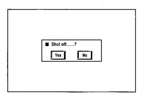
Press the Power (POWER) Key again, or move the high-lighted bar to [YES] by moving the Joystick then press the Joystick to execute the selection, to turn the systems power off except the AV Codec.
